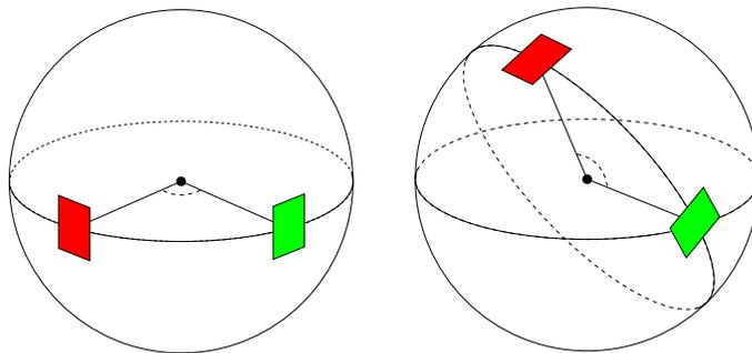
**Figure 1.** The key to global astrometry is to measure positions simultaneously in two fields separated by a large, fixed basic angle. By repeating this for a given field at different orientations (to give different reference stars) we can, in principle, determine absolute parallaxes.
