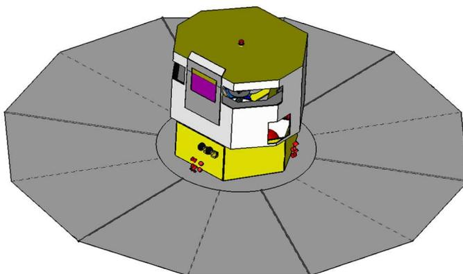
**Figure 4.** The Gaia satellite and sun shield. The payload module is 3.1m high and the sun shield has a diameter of 11m. Between the two entrance slits for the two astrometric fields at the top is the astrometric focal plane. © Astrium
