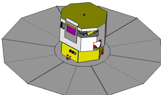
**Figure 4.** The Gaia satellite and sun shield. The payload module is 3.1m high and the sun shield has a diameter of 11m. Between the two entrance slits for the two astrometric fields at the top is the astrometric focal plane. © Astrium
