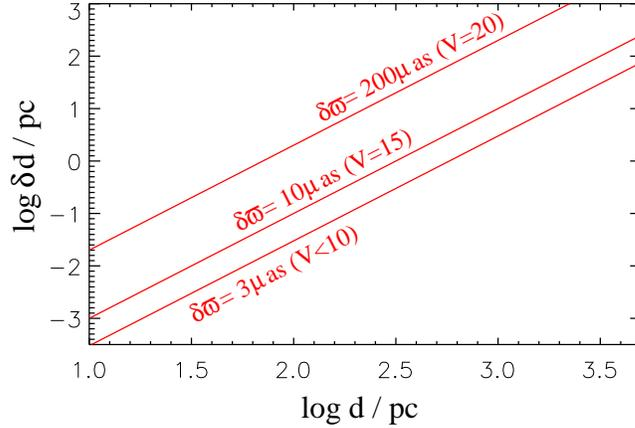
**Figure 6.** The Gaia distance accuracy at three magnitudes. To first order the uncertainty in the distance,  $d$ , is  $\delta d \sim d^2 \delta \varpi$ , where the parallax accuracy,  $\delta \varpi$ , depends only on the apparent brightness (to first order) as  $\delta \varpi \sim 1/\sqrt{N}$  ( $N$  is the number of photons collected).
