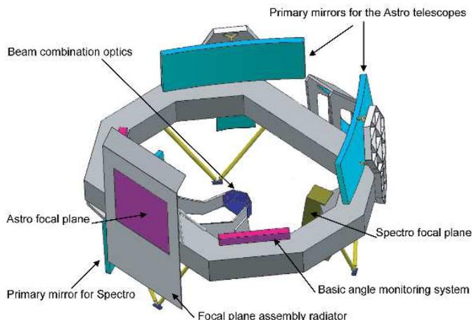
**Figure 5.** The Gaia payload. The two astrometric primary mirrors are  $1.4\text{ m} \times 0.5\text{ m}$  in size.
