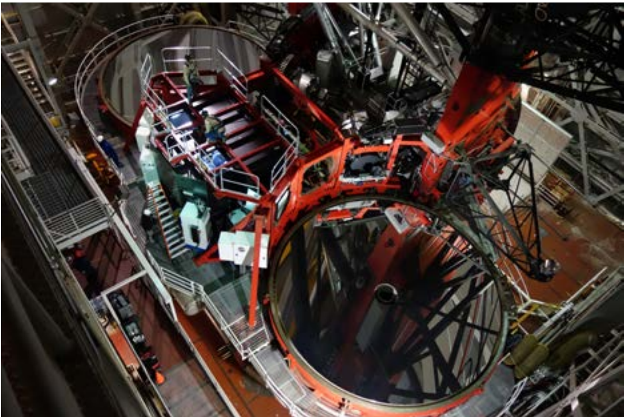
Fig. III.1.1: The Large Binocular Telescope (LBT) on Mount Graham in Arizona (USA). With its two 8.4 meter mirrors on a single mount, the LBT is currently the largest single telescope in the world with a total light gathering power of a 12 meter telescope. The image was taken during the test installation of the main LINC-NIRVANA structure, which
