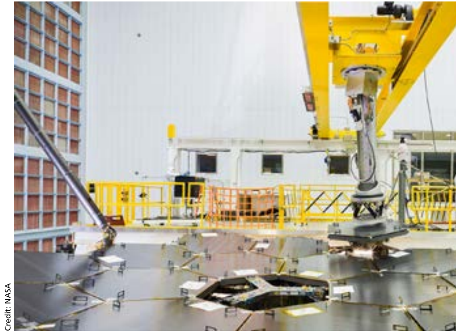
Fig. III.2.2: A close-up view of the eighteenth and final James Webb Space Telescope primary mirror segment being installed on the telescope. The black covers are protecting the gold-coated mirror segments.
