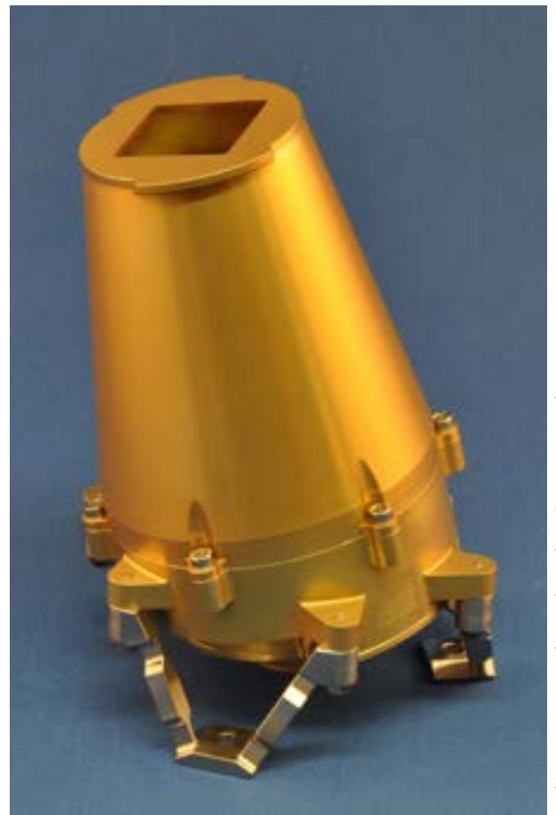
Fig. III.2.5: Structural and thermal model of the Euclid calibration source as delivered in December 2015 to the Laboratoire d'Astrophysique de Marseille (LAM) for installation as part of an instrument model.
