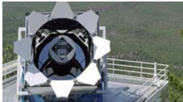
MPIA is a member of the Sloan Digital Sky Survey (SDSS), a spectroscopic survey using a 2.5 meter telescope in New Mexico. The survey gathers high-quality spectra of a large number of astronomical objects.
