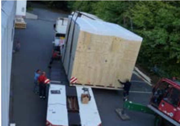
Fig. III.3.3: The LINC-NIRVANA optical bench begins its journey to LBT. Top left: Loading the large custom crate onto a "low-boy" transporter to enable safe passage under bridges and other obstructions. Top right: The late night trip from the Königstuhl to the Neckar river. Bottom left: Transferring the optical bench to the barge. Bottom right: The Venture with its single, large cargo item passes the old town of Heidelberg, heading for the North Sea.
