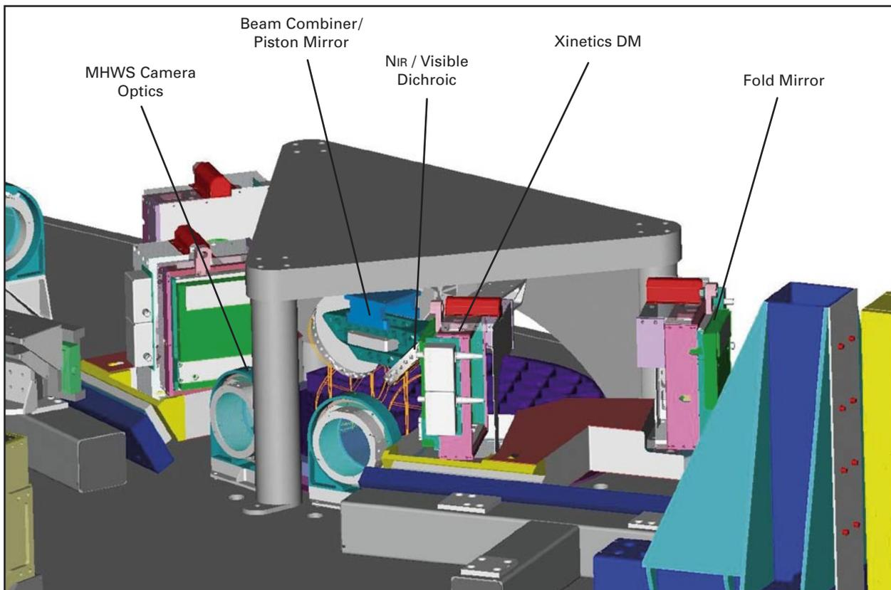
**Fig. IV.1.9:** Beam combination area, including Xinetics DMs, piston mirror, and the visible / near-infrared dichroic.
