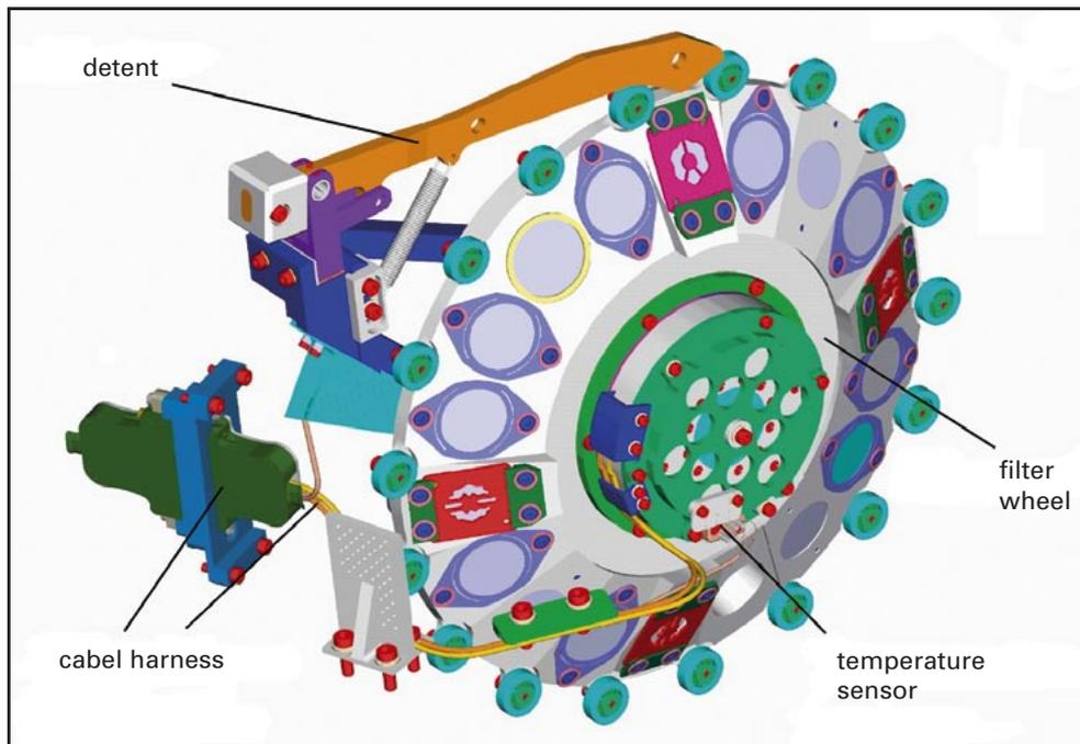
**Fig. IV.9.2:** The 18 positions of the MIRI filter wheel are equipped with broad- and narrow-band filters, coronagraphic masks and a prism for spectrophotometry. The center of the wheel harbors the direct drive; the index ball bearings and the detent are to be seen at the periphery of the wheel. The wheel is 25 cm across, the positioning accuracy is  $< 4$  arcsec.
