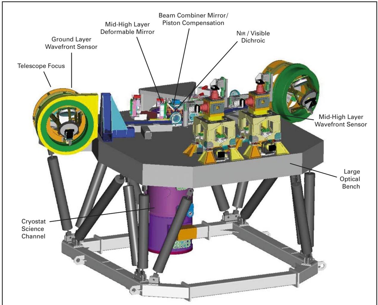
**Fig. IV.1.8:** Mechanical components associated with the LINC-NIRVANA optical path.
