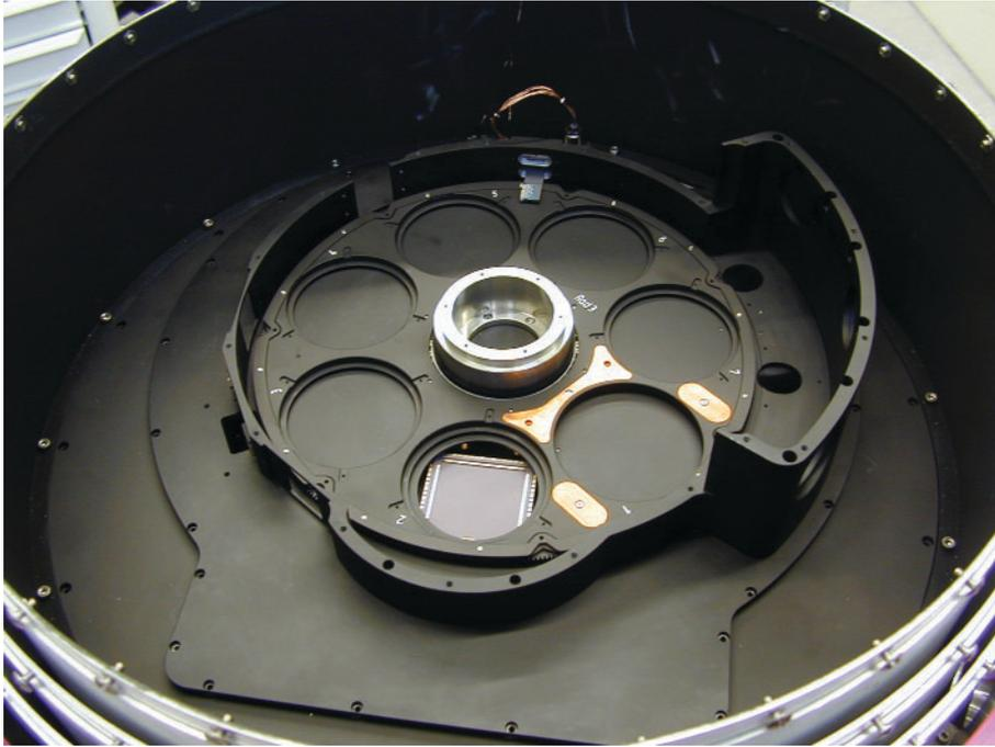
**Fig. III.5:** OMEGA 2000: **b)** view of the interior showing the filter wheel.
