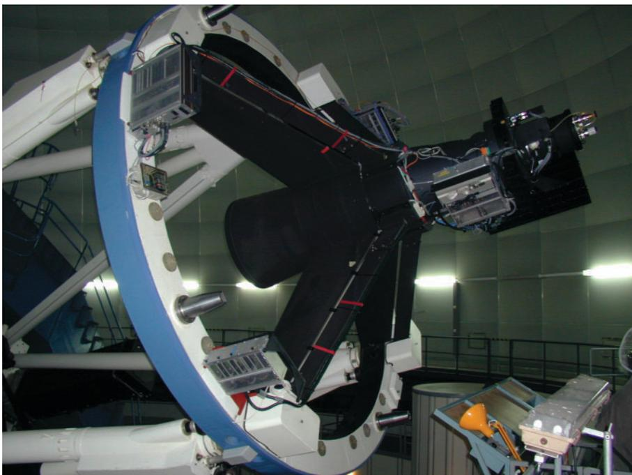
**Fig. III.6:** LAICA on the front ring of the 3.5m telescope on Calar Alto.
