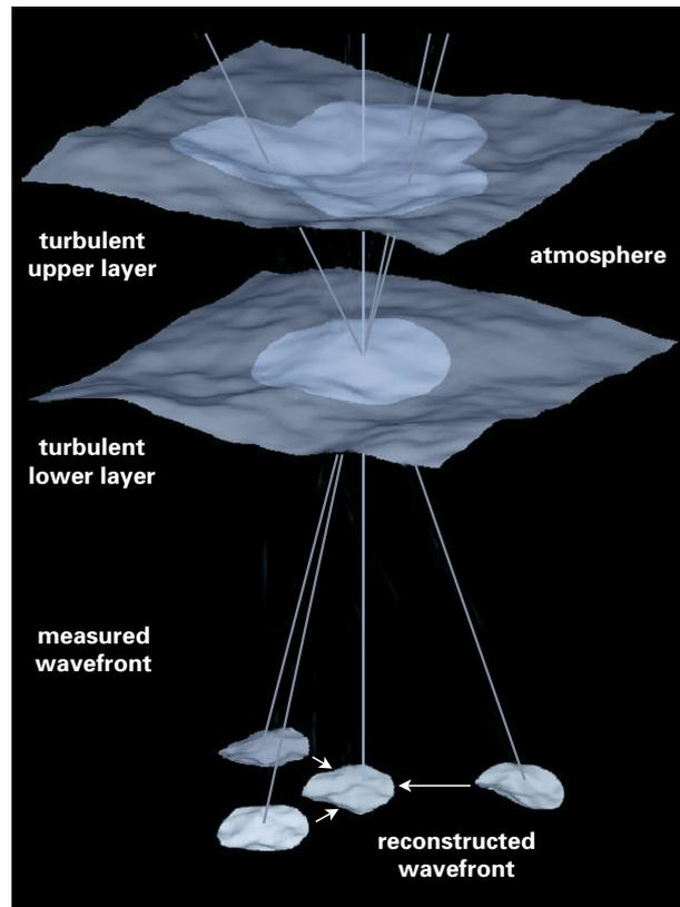
**Fig. III.3:** Disturbance of light rays coming from several directions in two atmospheric layers. From the measured wavefronts, the wavefront in the center, where the astronomical object is located, can be calculated.
