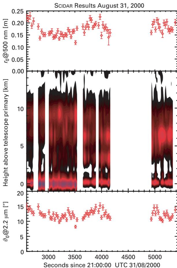
**Fig. III.2:** Characteristic results of SCIDAR measurements obtained at the Calar Alto Observatory. The values above and below indicate two important quantities of adaptive optics, the Fried parameter and the isoplanatic angle. In the middle, the turbulent structure of the atmosphere can be recognized.
