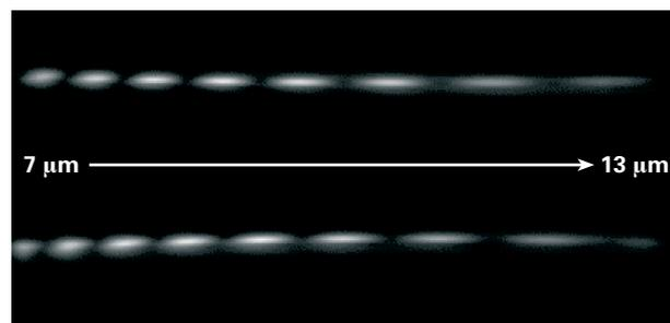
**Fig. III.7:** **a)** View of the interior of MIDI. The inner part of the optics is cooled by means of a closed cycle cooler (rear left at the instrument). Of the optical components, the filter wheel (black) is the most noticeable. **b)** Result of tests using a laboratory light source: interference pattern for wavelengths of  $7\ \mu\text{m}$  (left) to  $13\ \mu\text{m}$  (right).
