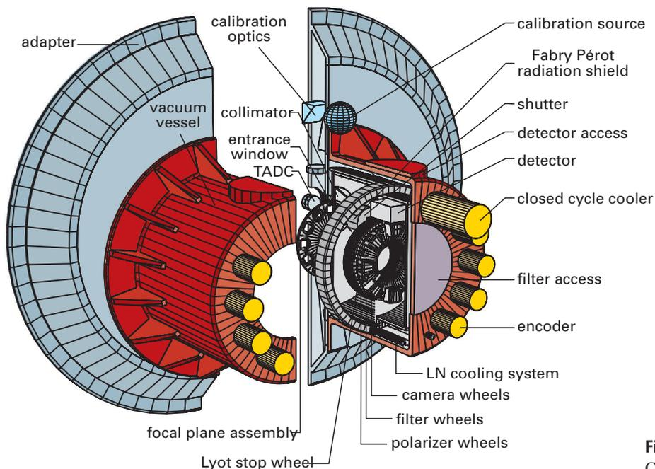
**Fig. II.3:** Conceptual overview of CONICA. (MPIA)
