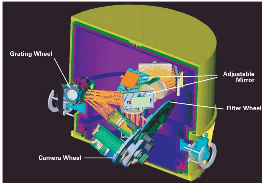
**Fig. III.11:** The optical and mechanical design of LUCIFER.
