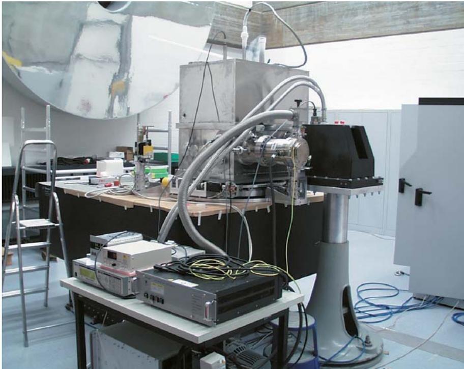
**Fig. III.9:** The cooling unit of MIDI during tests at the Institute.
