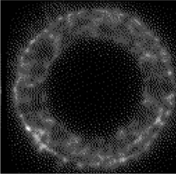
**Fig. III.1:** Pupil image of the 1.23 m telescope with SCIDAR. Intensity variations caused by diffraction effects within turbulent layers are seen (exposure time 1.3 ms).
