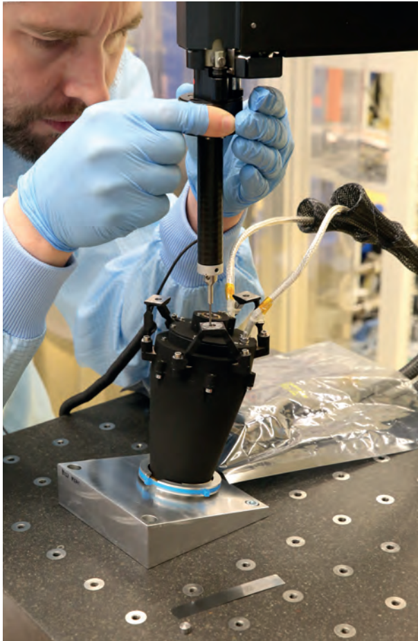
Fig. III.2.4: Final measurement of geometry and mounting interfaces for the NISP calibration lamp. Here the lamp is sitting upside down in the MPIA cleanroom for a measurement to confirm that the position of its six connecting legs are exactly as planned.
