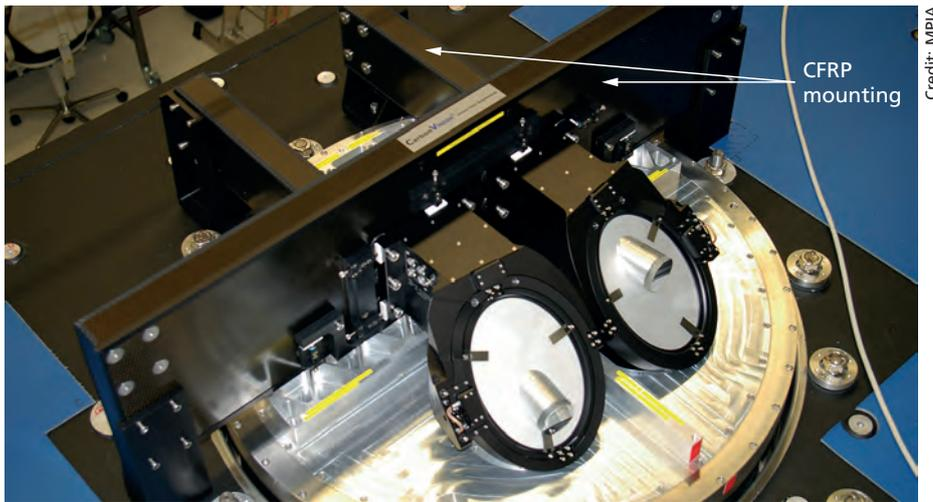
Fig. III.5.3: Structural components made of CFRP in the LBT instrument LINC-NIRVANA.
