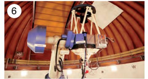
50 cm and 70 cm telescopes for testing and training purposes, here the 70 cm KING telescope.
