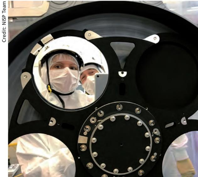
Fig. III.2.2: Final NISP photometric filter wheel in the process of being mounted inside the Flight Model. The wheel provides a closed shutter position (*black, right*), an open position, and three bandpass filters (*left top and bottom, right*). These only transmit light in the near-infrared and appear as mirrors in visible light, as in this picture, where the engineers are actually seen in reflection.
