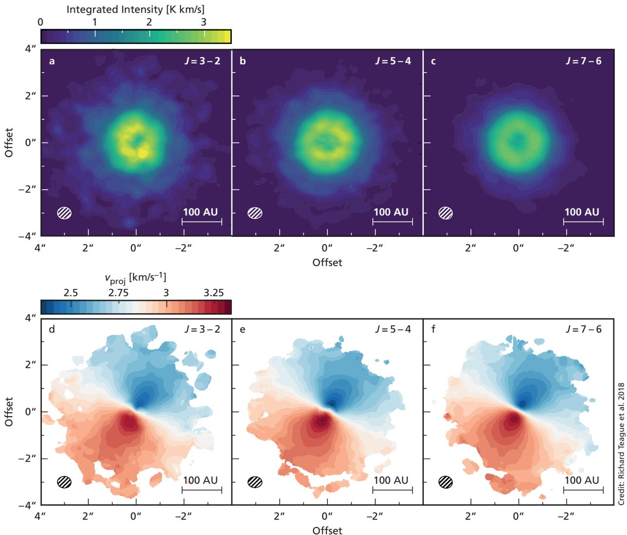
Fig. II.1.6: ALMA multi line observations in various CS transitions of the protoplanetary disk TW Hydrae. The top panel shows the integrated emission maps of the labeled transitions, and the bottom panels show the corresponding first moment maps (intensity-weighted peak velocities) outlin-
