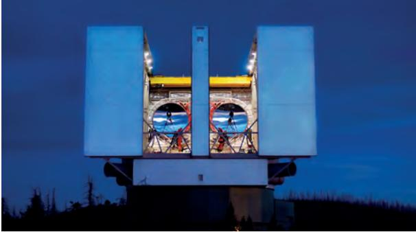
MPIA is part of the consortium operating the Large Binocular Telescope (LBT) on Mount Graham in Arizona. The LBT has two 8.4 meter mirrors on a single mount.
