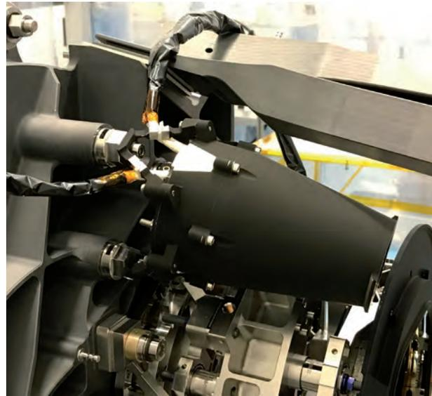
Fig. III.2.3: NISP calibration lamp NI-CU, provided by MPIA, as mounted in its final position on the NISP Flight Model. Clearly visible are the nominal and redundant harnesses, the cables providing power and diagnostic capabilities to the 2 x 5 LEDs inside the lamp.
