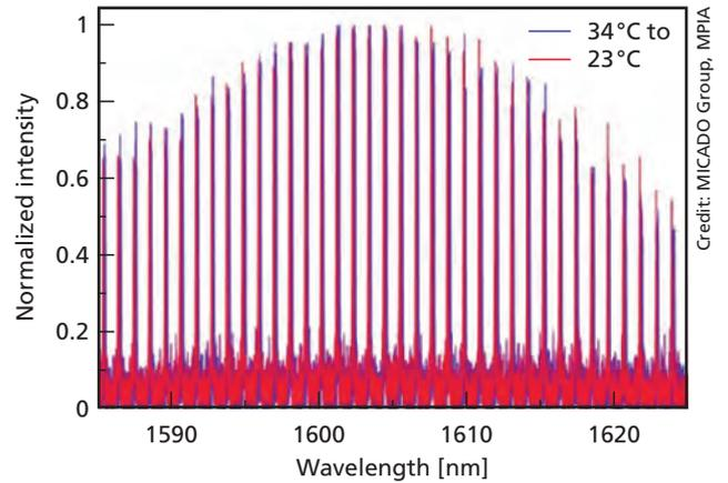
Fig. III.3.4: Measured spectrum from the prototype Fabry-Pérot under test at MPIA. A major concern of this device is its wavelength stability against temperature drifts.
