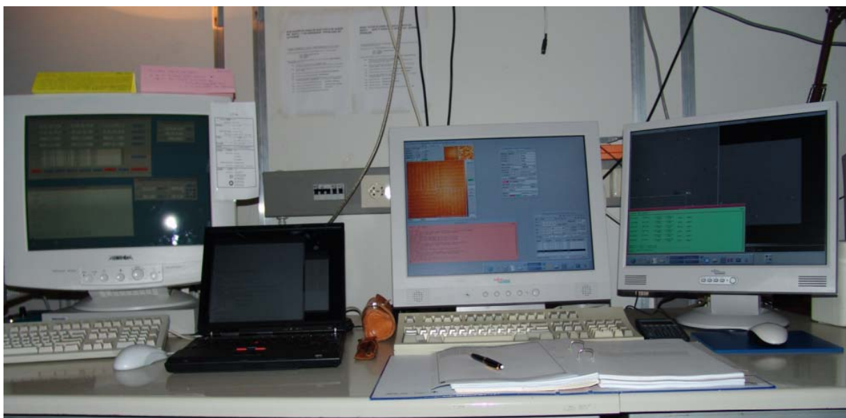
Figure 67: Dual-screen X-terminal (to the right) operates the camera. The screen at left is for telescope operation.
