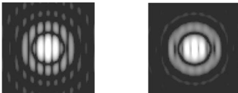
Fig. 6. Pupil signature of the PSF in case of a single exposure (left). For longer integration times the image of the PSF blurs due to the pupil rotation. The image on the right corresponds to about 30 degree of pupil rotation and illustrates the degradation of the angular resolution of about 10% along the horizontal center line.
