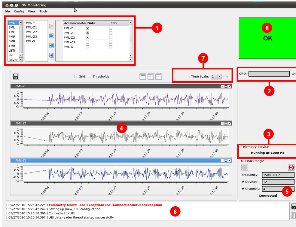
Figure 4. Preliminary version of the OVMS monitoring GUI. 1: Telescope component list. 2: OPD status. 3: Telemetry service status. 4: Vibration/PSD plots. 5: Data acquisition device status. 6: Logging window 7: Time range adjustment. 8: Threshold alarm.
