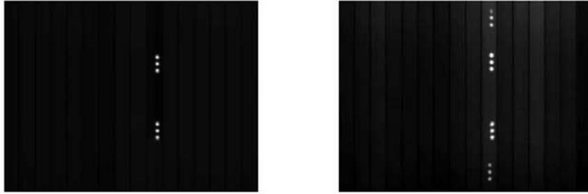
Figure 3. Detector images taken in two different observing modes: ‘High Sens Mode’ (left) with only the two interferometric output channels and ‘Photometric Mode’ (right) with two additional photometric channels. Every channel shows an image of the triple pinhole used here. Slits have the same orientation as the triple pinholes.
