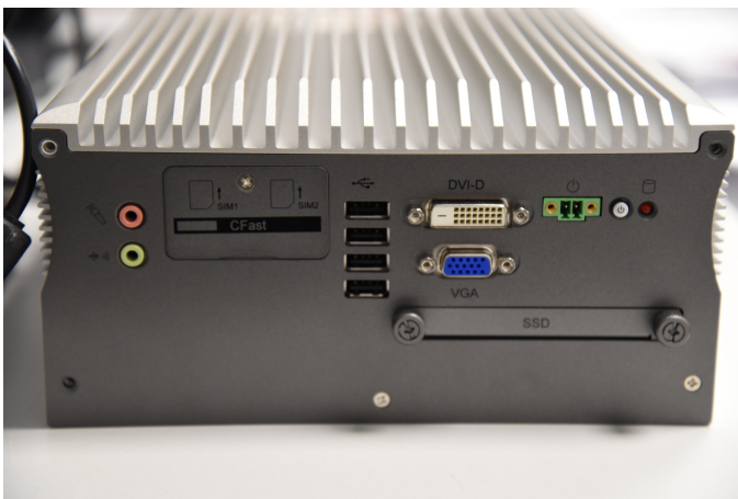
Figure 9: Front of the PicoSys 2614 computer. The current setup is that the two monitors are connected to the display ports (DP) on the rear side, and mouse and keyboard with two of the four USB ports at the front side.
