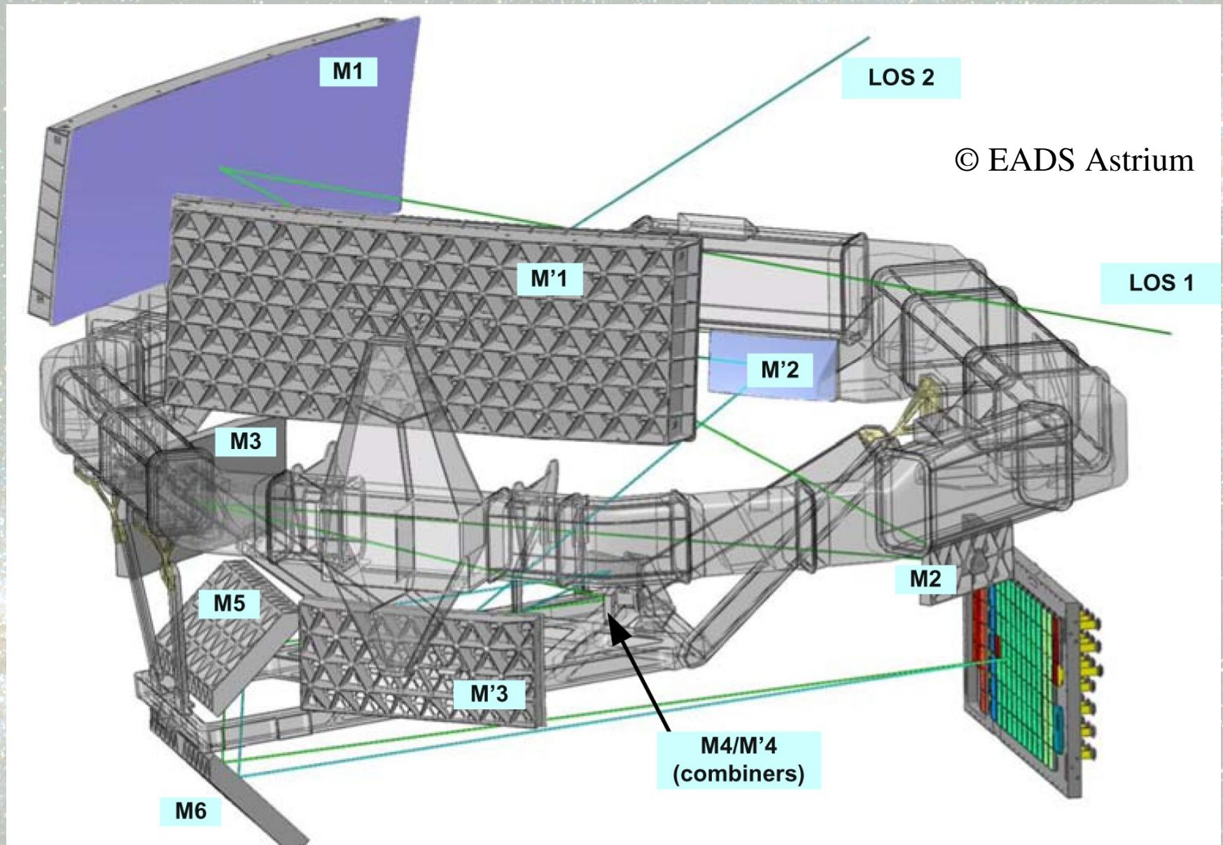
Two fields-of-view superimposed on a common focal plane
