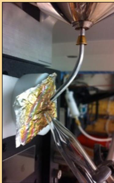
Soft ionization method (no fragmentation) operating at atmospheric pressure and ambient conditions.
