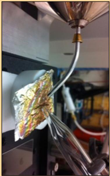
Soft ionization method (no fragmentation) operating at atmospheric pressure and ambient conditions.
