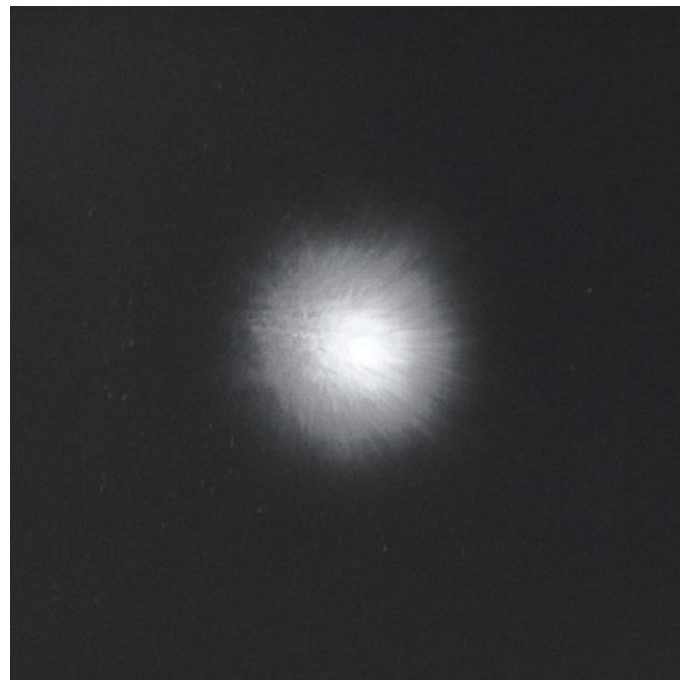
Fig. III.2.5.: The same star, but now after activation of the adaptive optics. Although this picture was taken during 2.3 arcsecond seeing (which indicates very bad turbulence) and in visible light (where adaptive optics never works well – the LN camera will operate at infrared wavelengths), it shows a dramatic improvement in sharpness and intensity.
