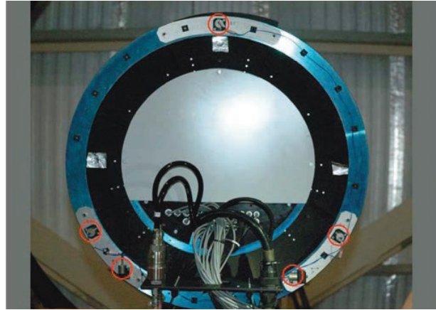
Fig. III.2.8: Five vibration sensors on the mount structure of one of the two adaptive secondary mirrors of the LBT.
