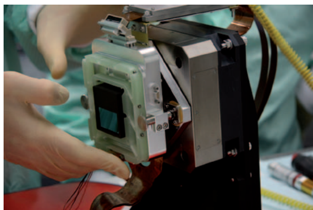
Fig. IV.3.1: The detector motion stage with the engineering grade detector, being mounted for the first time into the IRDIS system.
