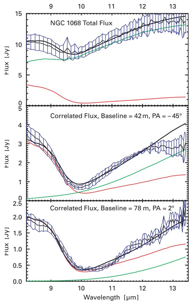
**Fig. II.23:** Spectra of NGC 1068, obtained with MIDI. The cross-hatching indicates the measurements with their uncertainty, the solid line shows values for a model. The red and green lines show the contributions of the hot and warm components, respectively. Top: Single-telescope spectrum with the characteristic silicate absorption feature at 10  $\mu\text{m}$ . Middle: Interferometrically “magnified” spectrum at 0.026 arcseconds resolution; bottom: the same at 0.013 arcseconds.
