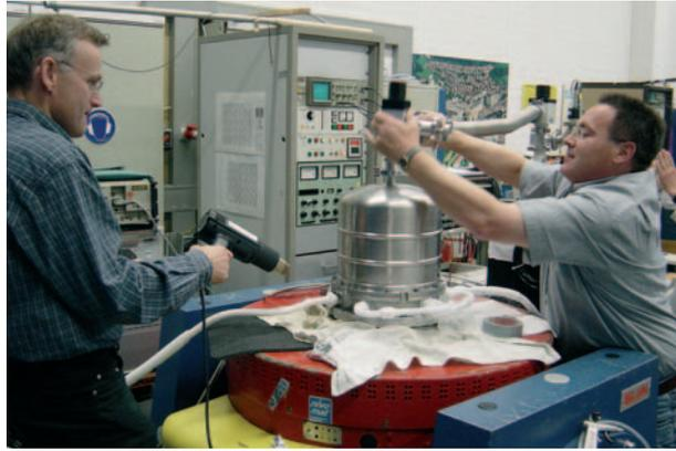
**Fig. IV.19:** Cold vibration test of the focal-plane chopper for PACS in the cryostat on the vibration table at C. ZEISS .
