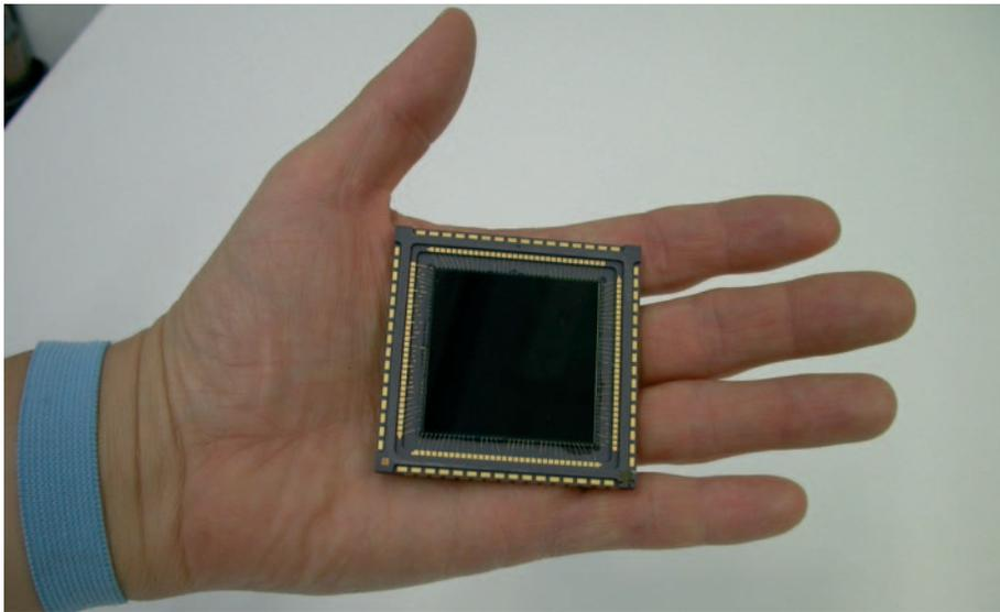
**Fig. IV.2:** The detector for the infrared camera OMEGA 2000
