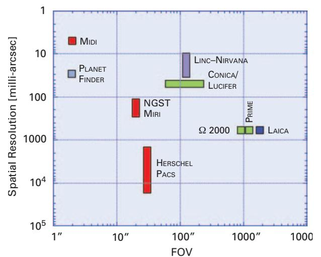
**Fig. I.7:** The Institute's major instruments. Spatial resolution as a function of the field of view.
