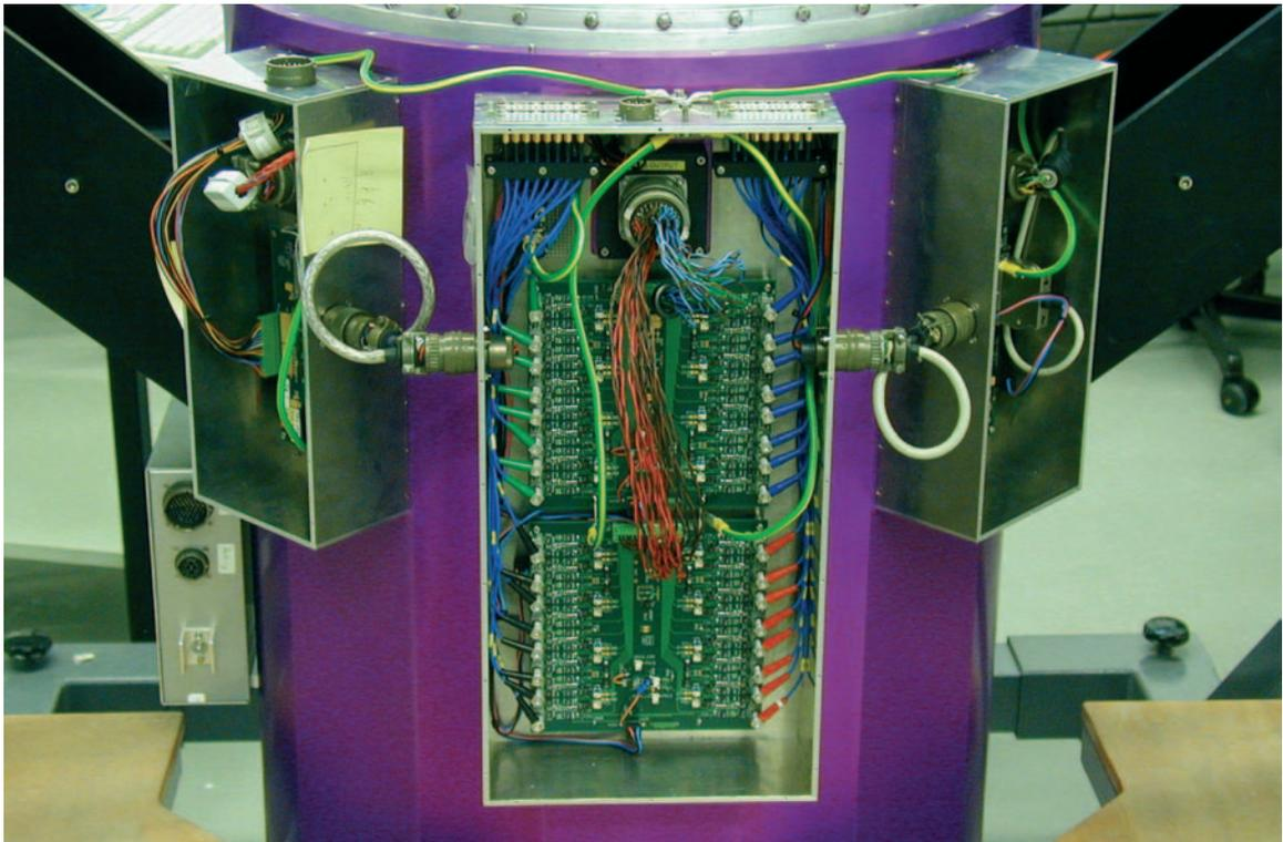
**Fig. IV.4:** Control and read-out electronics of the infrared camera.
