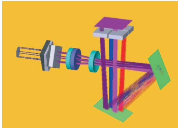
**Fig. IV.17:** Supplement of the CONICA optics for observations in the SDI mode. Major components are the two Wollaston prisms, the lens system and the quadrant filters.
