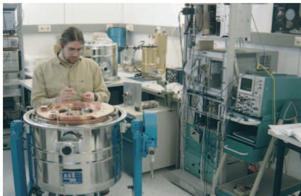
**Fig. IV.21:** The Ge:Ga detector arrays for PACS are installed in the test chamber at MPIA.
