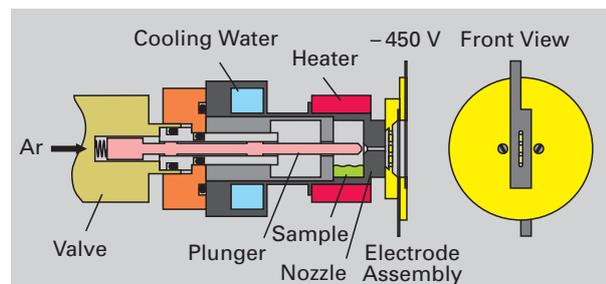
**Fig. III.10:** Schematic view of the pulsed supersonic jet source. The PAH molecules are contained in the sample in a crystalline form. The electrode assembly is only installed when PAH cations are to be studied.
