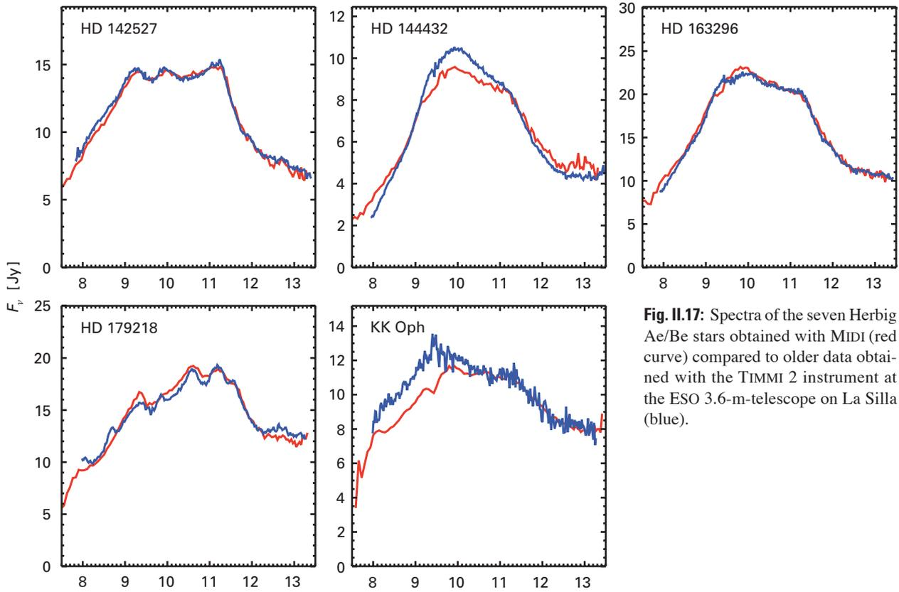
**Fig. II.17:** Spectra of the seven Herbig Ae/Be stars obtained with MIDI (red curve) compared to older data obtained with the TIMMI 2 instrument at the ESO 3.6-m-telescope on La Silla (blue).
