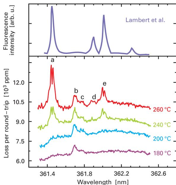
**Fig. III.12:** CRD spectra of the neutral anthracene molecule taken in the expansion of a supersonic jet on the red side of the  $0 \leftarrow 0$  band for different nozzle temperatures. For comparison with the absorption measurements, the upper frame shows a LIF spectrum obtained by Lambert et al.
