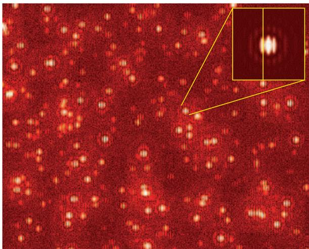
**Fig. IV.14:** Simulated image of a star field as seen by the LINC-NIRVANA instrument. The insert image shows the interferometric fringe pattern that is folded into each object image in the instrument field of view.
