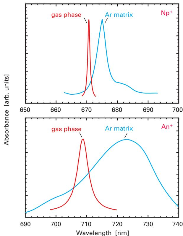
**Abb. III.13:** Gas phase absorption spectra of naphthalene ( $\text{Np}^+$ ) and anthracene ( $\text{An}^+$ ) cations (red curves) taken with CRDS in comparison to Ar-matrix data (blue curves).
