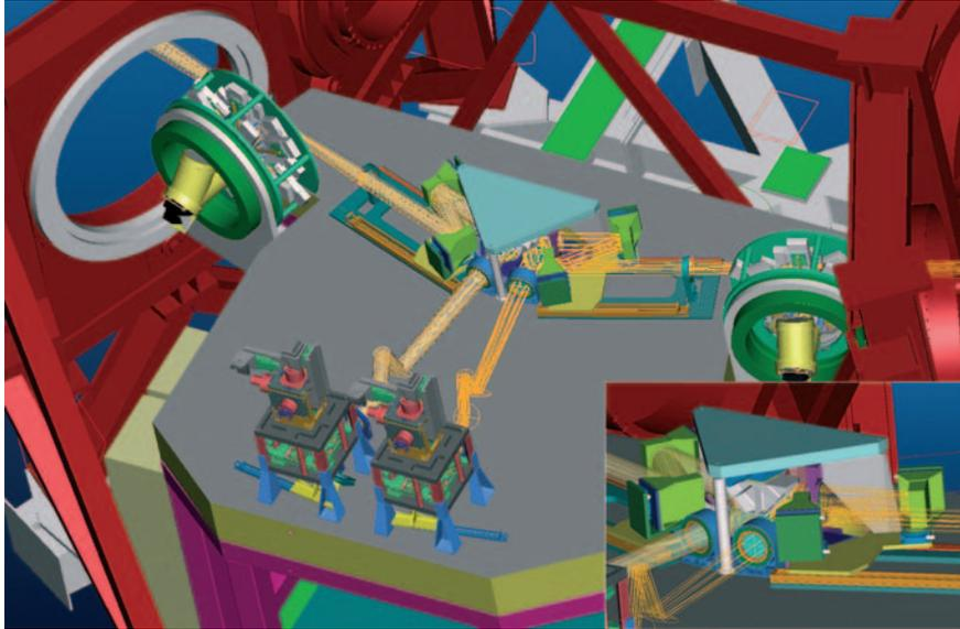
**Fig. IV.12:** Overview on the light path at the optical bench of LINC-NIRVANA. The insert image shows the ‚crowded area‘ of the piston mirror that is located in the center of the overview image.
