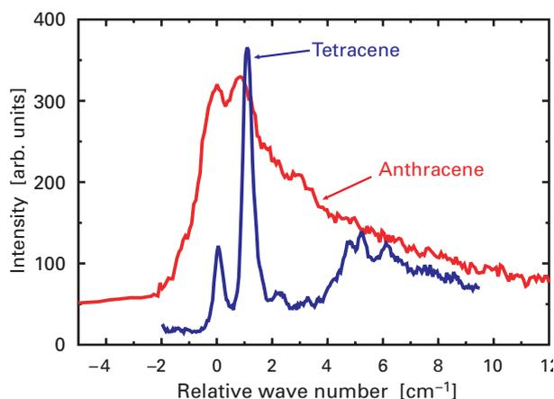
**Fig. III.17:** LIF-spectra of the PAH molecules anthracene and tetracene in helium droplets.
