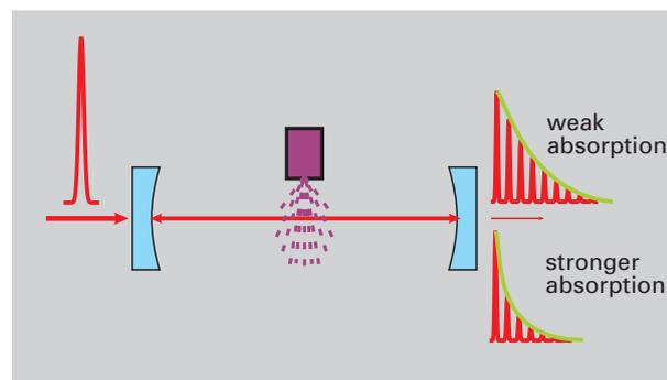
**Fig. III.11:** Principle of the cavity ring-down spectroscopy (CRDS).
