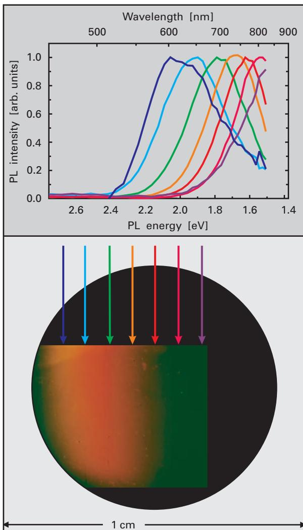
**Fig. III.22:** Photoluminescence curves of Si nanoparticles of various sizes deposited on a substrate after size selection in the molecular beam. The photo below shows the luminescent layer of the Si nanoparticles after excitation with a UV light source.
