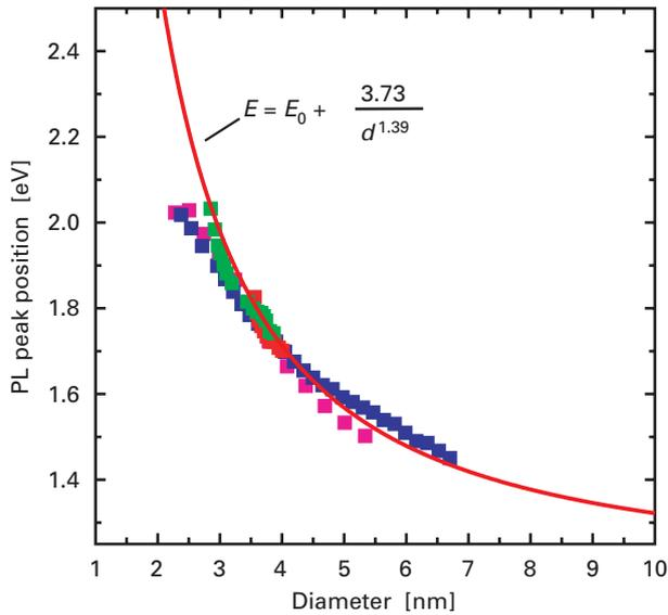
**Fig. II.23:** Theoretical correlation between the position of the PL maximum and the size of the silicon nanoparticles (red curve) compared to experimental data obtained from various samples.
