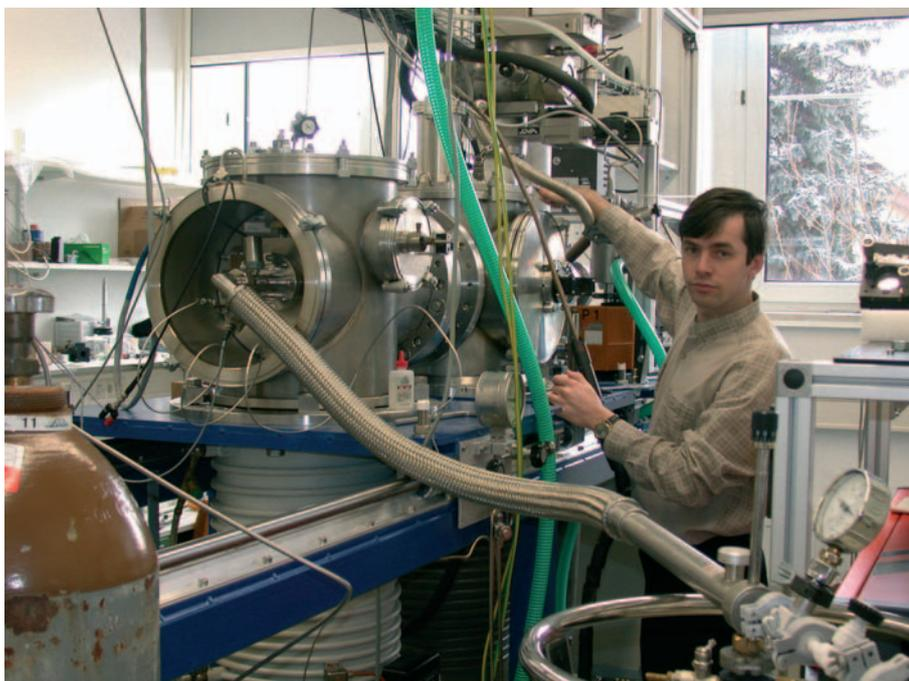
**Fig. III.19:** Molecular-beam apparatus used to produce and spectroscopically characterize the helium droplets with embedded PAH molecules. Serge Krasnokutski tightens the last screw before evacuating the chambers. The hose seen in the foreground conveys the liquid helium used for cooling the nozzle.
