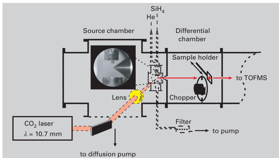
**Fig. III.20:** Schematic representation of the molecular beam apparatus for production, selection and size determination of silicon nanoparticles.
