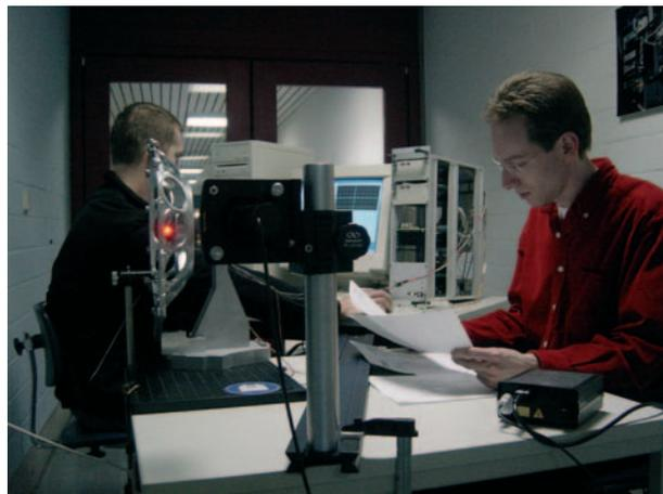
**Fig. IV.24:** The prototype of a filter wheel for NIRSPEC is tested at MPIA with regard to the dependence between achievable position accuracy and electric power dissipation.
