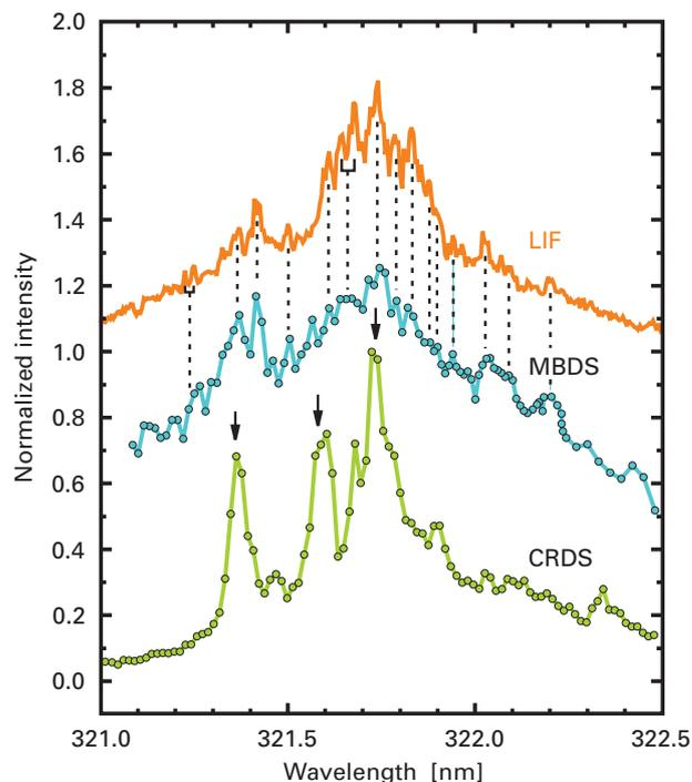
**Fig. III.18:** Three absorption spectra of the pyrene molecule, measured in He droplets with the LIF as well as the depletion method (MBDS) and in the gas phase (CRDS). The CRDS spectrum was shifted by 0.8 nm towards longer wavelengths.
