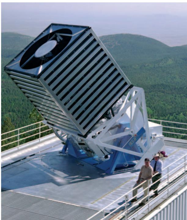
**Fig. III.32:** The 2.5-meter telescope of the Sloan Digital Sky Survey, located in the Sacramento Mountains of southern New Mexico in the United States. The box-like structure protects the telescope from being shaken by the wind.
