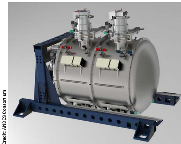
Fig. IV.4.3: ANDES K-band spectrograph cryostat design presented in the subsystem review in November 2024.
