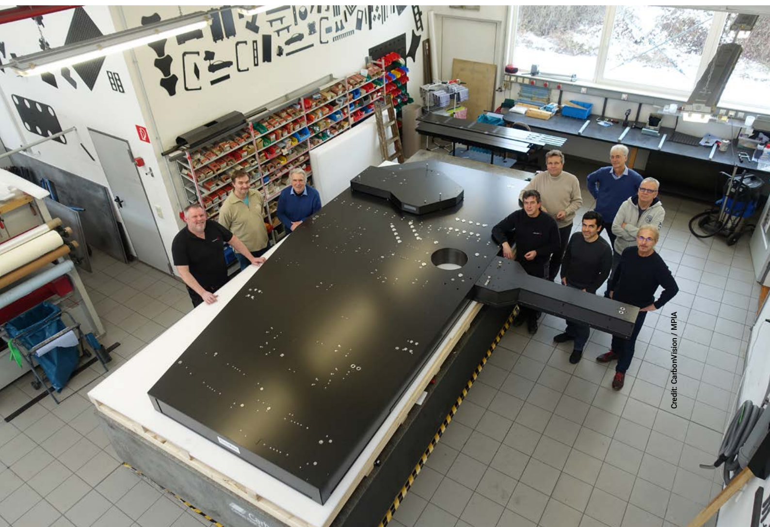
Fig. IV.1.2: MICADO's carbon fiber optical bench, manufactured by CarbonVision, that will hold its relay optics. The picture shows parts of the CarbonVision and MPIA teams at the acceptance of the bench in the CarbonVision facilities.
