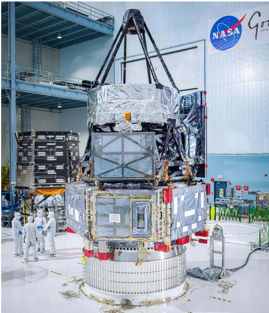
Fig. IV.2.1: Roman Spacecraft Integrated Payload Assembly in the cleanroom at NASA's Goddard Space Flight Center in December 2024. The telescope is mounted on top of the instrument carrier with both the CGI and WFI instruments.
