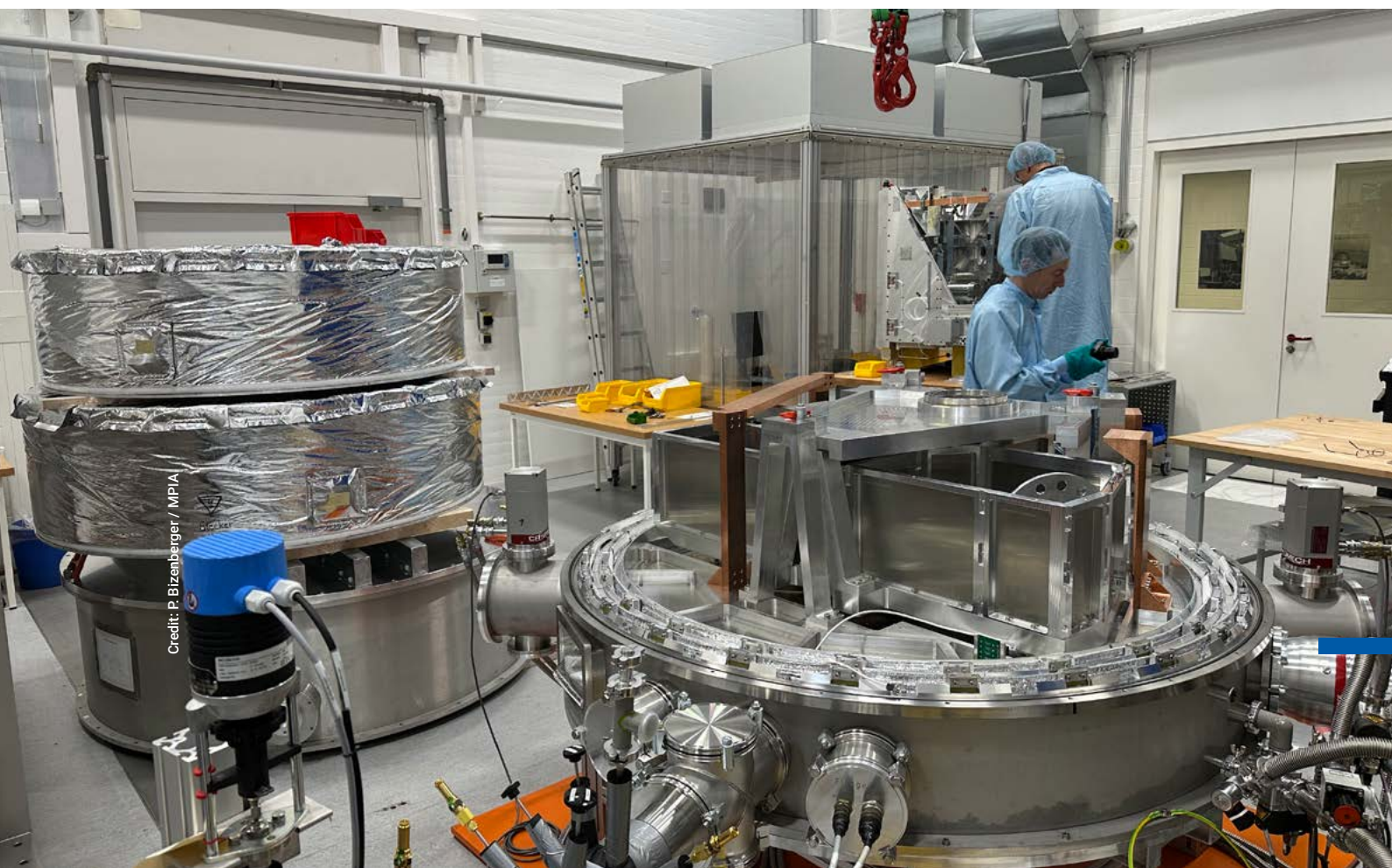
Fig. IV.5.2: METIS adaptive optics unit test setup being assembled at MPIA.
