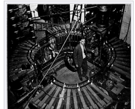
The first synchrotron to use the "racetrack" design with straight sections, a 300 MeV electron synchrotron at
